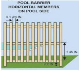
6. Where the barrier is composed of horizontal and vertical members and the distance between the tops of the horizontal members is 45 inches or more (1143 mm), spacing between vertical members shall not exceed 4 inches (102 mm). Where there are decorative cutouts within vertical members, the interior width of the cutouts shall not exceed 1¾ inches (44 mm) (305.2.6)
